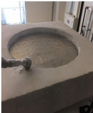
LN2 bucket for test cryostat. Zotefoam bucket + HR-25 + Aluminum Plate
