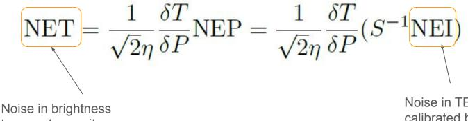
temperature units (per rt[integration second]) Noise in TES current calibrated by readout resistances (per 1/rt[Hz] bandwidth)
